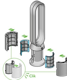
The air purifier with the filter covers open showing a HEPA plus carbon filter located in the filter covers and a catalytic filter. Arrows demonstrate that the catalytic filter is fitted directly to the base of the machine and the filter covers will need to be assembled onto the base of the machine.
