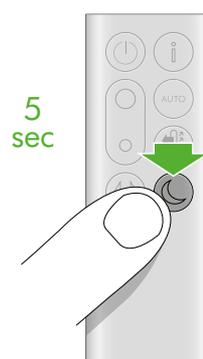
Pressing the night mode and sleep timer button on the bottom right of the remote control for 5 seconds.
