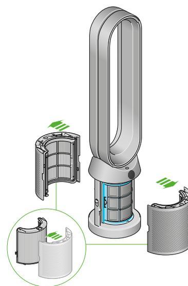
The air purifier with the filter covers open showing a HEPA filter located in the filter covers and a carbon filter. Arrows demonstrate that the carbon filter is fitted directly to the base of the machine and the filter covers will need to be assembled onto the base of the machine.
