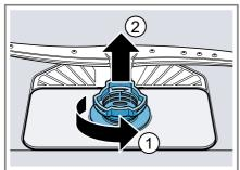
Pull down the micro filter to remove.
