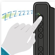
3 Slowly move your finger one or two mm away from the needle at the bottom of an ion optic. You will hear a slight sizzle. It is possible to see a glow at the tip of the needle if your room is dark enough.
