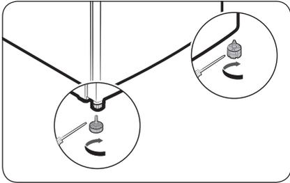
Level the refrigerator by manually adjusting the levelling feet.
