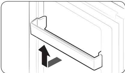
Slightly lift up and pull out the door bin.
