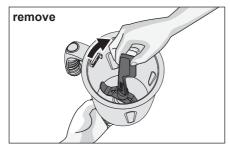
2. If the coupler is removed (the blade sticks together with the axis), washers will come off when you take blade assembly out of the jar.
