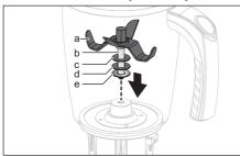
Put 2 x fibre- and metal washer onto the axis from the underside and tighten the coupler by rotating it in an anti-clockwise direction.
