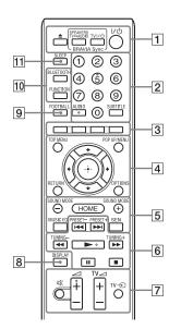
Number 5, AUDIO, ∠ +, and ► buttons have a tactile dot. Use the tactile dot as a reference when operating the remote control.
