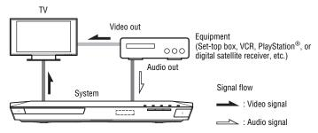
Select one of the following connection methods according to the jack type of the equipment.
