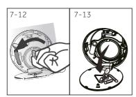
Scalding Risk! Water in the pump filter can be very hot! Before any action please ensure water has cooled down.
