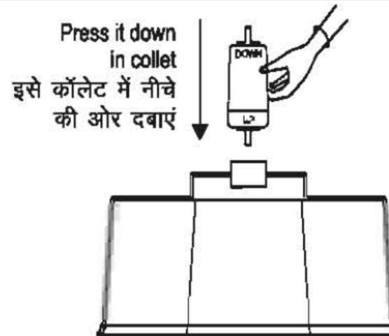
Push-fit the new membrane cartridge into the top tank
