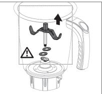
Hold the blade assembly with cloth. Using spatula untighten the blade nut (turn in a clockwise direction).
