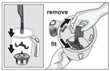
**Note:** If the coupler and/or some other parts are removed during removing the blade, please refer to  $\rightarrow$  *"Blade changing procedure" see page 9.*
