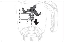
7. Put 2 x fibre- and metal washer onto the axis from the underside and tighten the coupler by rotating it in an anti-clockwise direction.
