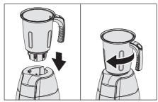
3. How to fit/remove active flow breaker Your Bosch TrueMixx Mixer Grinder has an active flow breaker which improves the quality of your wet grinding applications. To fit the active flow breaker, insert the active flow breaker in the groove on the inside surface of the big jar and slide it in until it fits properly. To remove it, gently press in the opposite direction till it disengages. Slide it out thereafter.
