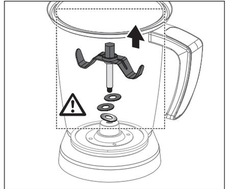
4. Hold the blade assembly with cloth. Using spatula untighten the blade nut (turn in a clockwise direction).
