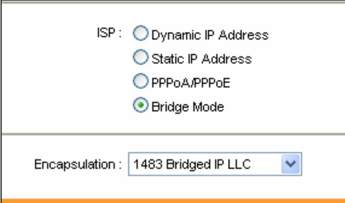
The screenshot shows a configuration window for the Internet Service Provider (ISP). It contains four radio button options: 'Dynamic IP Address', 'Static IP Address', 'PPPoA/PPPoE', and 'Bridge Mode'. The 'Bridge Mode' option is selected, indicated by a green dot. Below these options is a section labeled 'Encapsulation:' with a dropdown menu currently set to '1483 Bridged IP LLC'.
