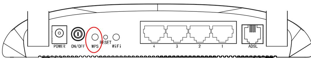
**Step 2:** Press and hold the WPS button of the adapter directly for 2 or 3 seconds.
