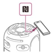
Complete the connection by following the instructions displayed on the BLUETOOTH device. When the BLUETOOTH connection is established, the BLUETOOTH device name appears on the display.
