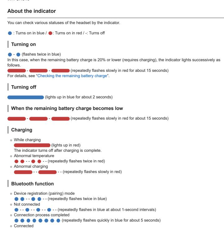
The not connected and connected status indications automatically turn off after a period of time has passed. They start flashing again for a period of time when some operation is performed. When the remaining battery charge becomes low, the indicator (red) starts flashing.
