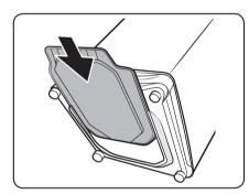
The washing machine comes with the Antirat panel that protects small animals such as rats from entering the machine. Insert the panel into the bottom of the machine. To facilitate the work, slightly lift up the bottom front.
