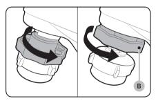
**3.** When levelling is complete, tighten the nuts (B) if provided (some models may not have the nuts).
