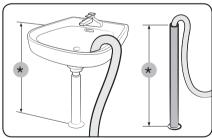
2. Connect the other end of the drain hose to a standpipe or basin that is positioned 90-100 cm (\*) from the floor.
