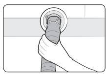
2. Insert the drain hose into the drain outlet. Make sure to connect them firmly using the joint ring.
