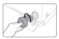
**1.** Put a floor-cloth or towel under the Pump filter. Turn the filter knob anticlockwise to remove.
