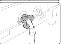
**3.** Reinsert the filter. Make sure it is tightened against water leaks.
