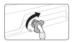
**7.** Connect the other end of the water hose to the inlet valve on the back of the washing machine. Turn the hose clockwise to tighten.
