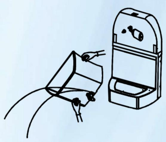
To keep the storage tank clean, it should be removed, drained and wiped dry, once in 15 days.
