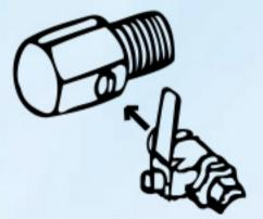
4. Attach the threaded end of the 3-way connector to the raw water supply and plug off the other end or connect to a tap.
