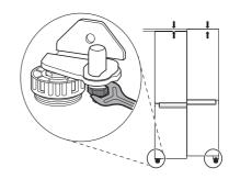
1 Open the door and use the spanner 1 to loosen the keeper nut by turning it to the left.
