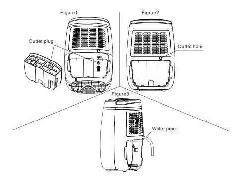
Note: Smoothly stretch the drainage, for if it is flat or twists together, drainage will not go on right; even the unit can not work normal. During the operation drainage pipe should never be in higher position than the hose connector.
