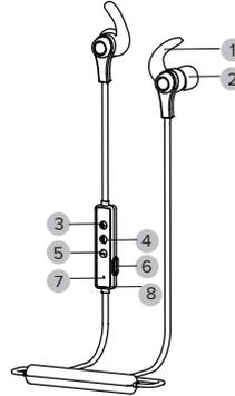
3. **Charging:** When charging, a red LED light will illuminate. The light will turn off when your unit is fully charged. Your headphones can take up to one hour to fully charge.
