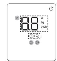
**01** Temperature indicator (numeric) Filter reset indicator (**F**) Electricity consumption indicator (numeric) (For AR\*\*CYNZ\*\*\*\*, AR\*\*CY4\*\*\*\*, AR\*\*CY5\*\*\*\*\*. AR\*\*CYMZ\*\*\*\* models) Auto clean indicator ([ 1)
