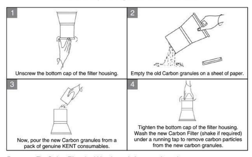
Frequency: The Carbon Filter should be changed after every 6 months.
