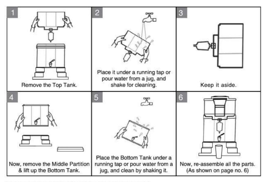
Frequency: Both water tanks must be cleaned once a week.
