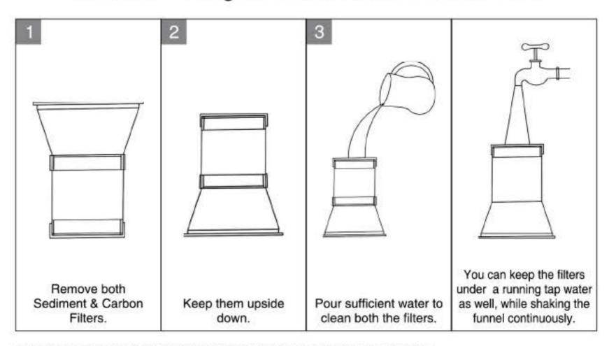
Frequency: Both Sediment & Carbon Filters must be cleaned once a week.
