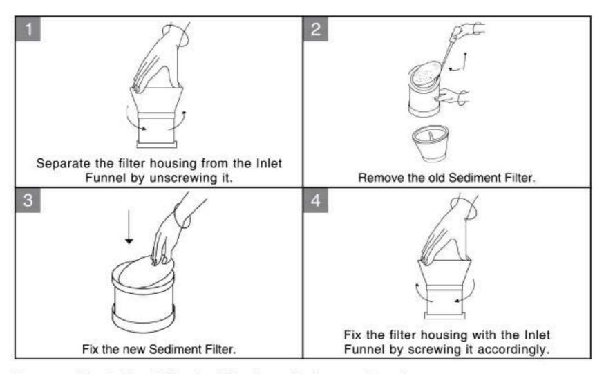
Frequency: The Sediment Filter should be changed after every 3 months.
