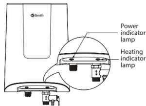
Switch on the Water Heater's power supply. The Power indicator lamp glows.
