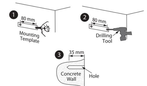
1. Insert the Expansion anchor into the hole (Step 1).
