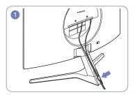
Connect cables to their port and route them through the ring on the Push the cables further close to the stand. back of the stand.
