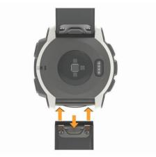
**NOTE:** Make sure the band is secure. The latch should close over the watch pin.
