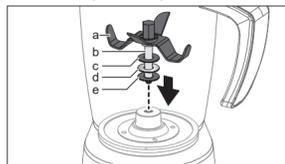
7. Put 2 x fibre washer and metal washer onto the axis from the underside and tighten the coupler by rotating it in an anti-clockwise direction.
